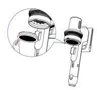
Clean dust cup and filters with water. Make sure that the dust cup and filters have dried before use.
