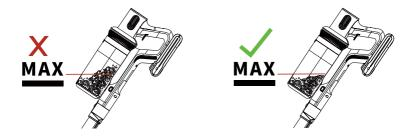
Press the dust empty button to empty the dust.
