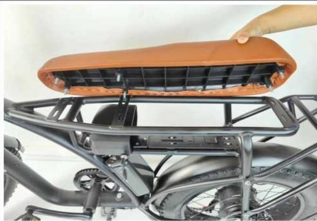
Put the saddle on the frame
