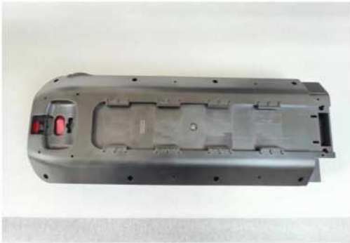
The switch of the battery is on the bottom
