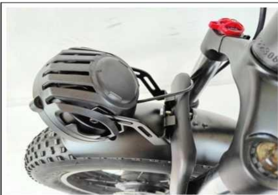
Use the long bolt to join the headlight, fork arch and fender
