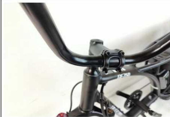
Handlebar installation completed
