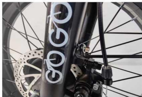
Fix the fender sticks to the fork
