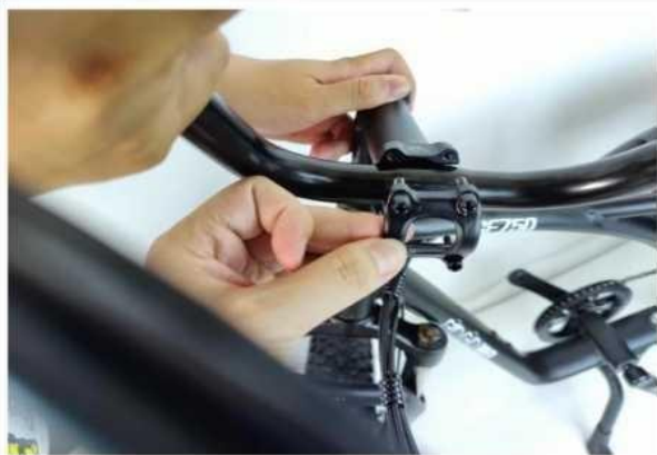
Tighten the 4 bolts
