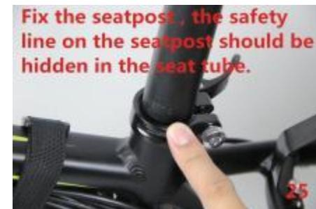
**Adjust the height and then lock the seatpost**
