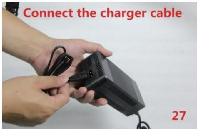
**Connect one side of the charger to the battery**
