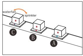
C.Waterfall/Sprinkler transferable switch(Marked with Icon) B.Controls the water inflow and the water temperature: Up the handle to open, otherwise down the handle to close water inflow (You pull up the handle higher; the water force will be stronger. Otherwise, the water force will be weaker.);
