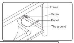
The bathtub must be connected to the ground. Power outlet must be sealed well. Make sure the surface of each wire is intact.
