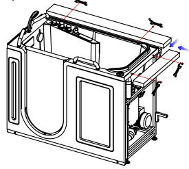
Connect your drain hose and the floor drain
