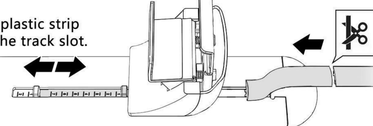
Cut the rubber strip to the desired length and insert into the track slot.
