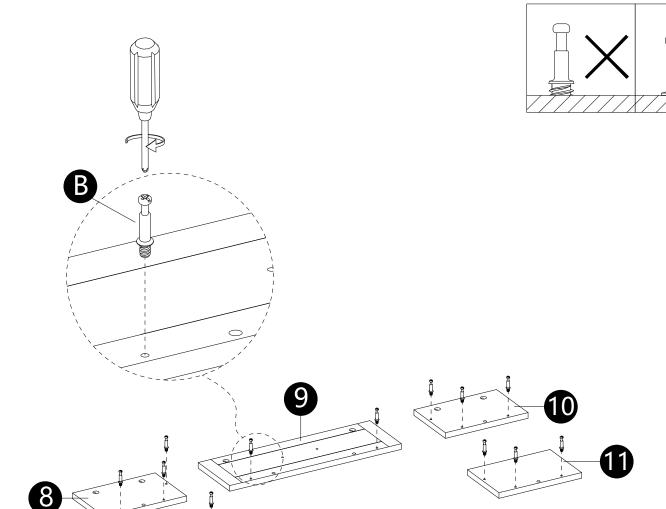
· Screw Cam bolts (B) into panels (8,9,10,11,12).
