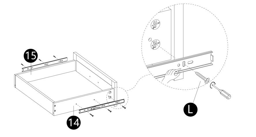
· Attach slider brackets to panels (14,15) with screws (L) correctly.
