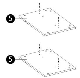
· Screw Cam bolts (B) into panels (4,5).
