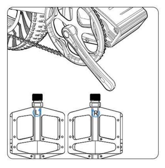
17. Identify the left (L) and right (R) pedals the left and the right pedals are marked on both ends.
