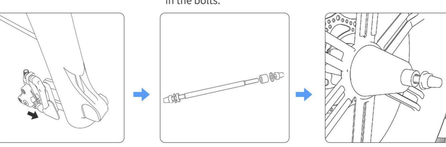
4. Release the front brake by removing the plastic spacer.
