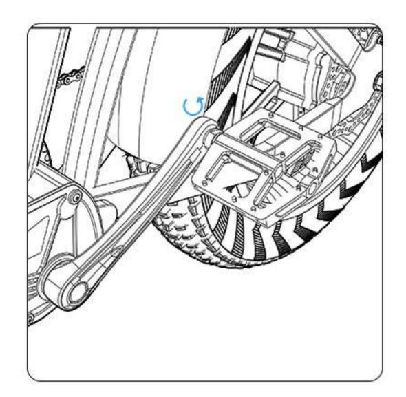
19. Install the left pedal by tightening the pedal in a counterclockwise direction.
