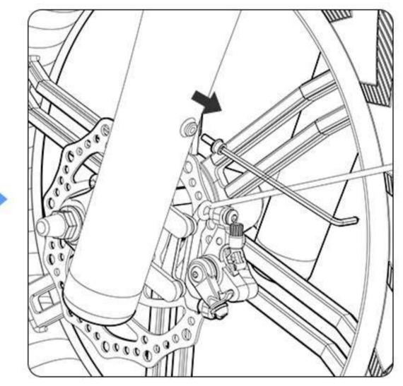
12. Remove the fender brace mounting hardware from the legs of the front fork.
