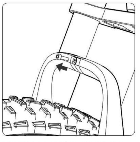
10. Remove the mounting hardware from the arch of the fork.
