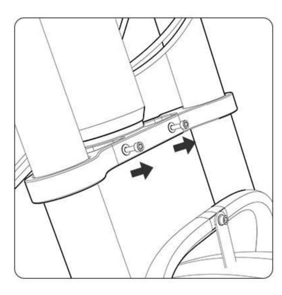
14. Remove the headlight mounting hardware from the crown of the fork.
