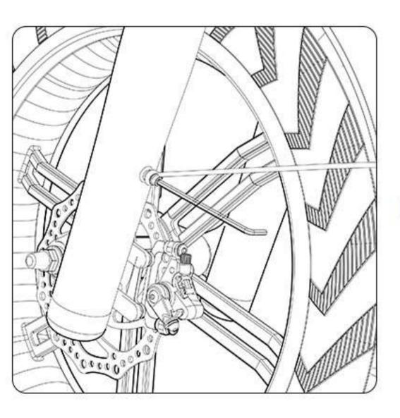
13. Pass the bolts through the steel spacer, then fender arm eyelets. Use a 4mm Allen key to tighten the bolts.
