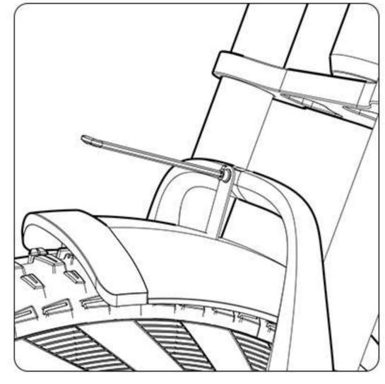
11. Fully tighten the nut by using a 5mm Allen key.
