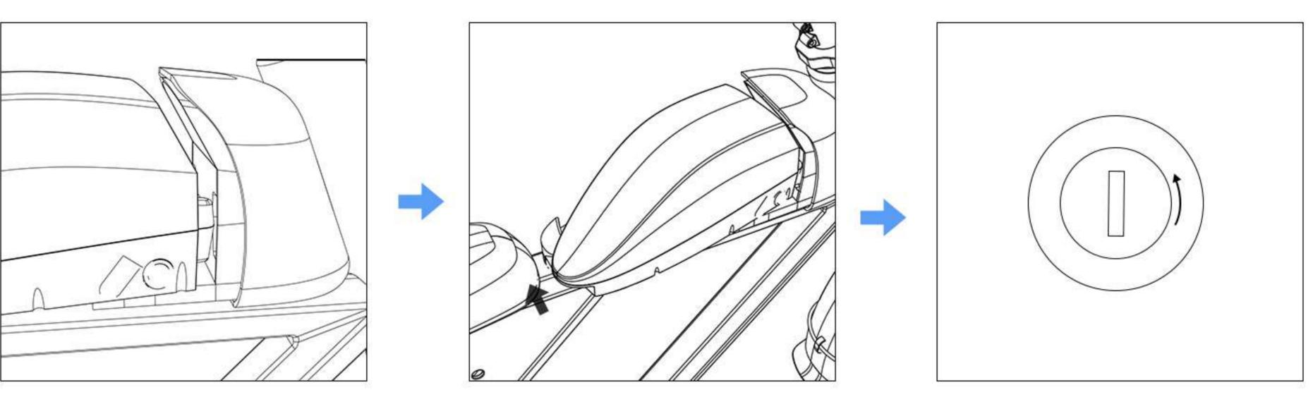
Install the battery with the contacts side forward.
