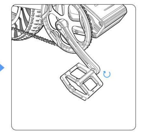
18. Install the right pedal by tightening the pedal in clockwise direction.
