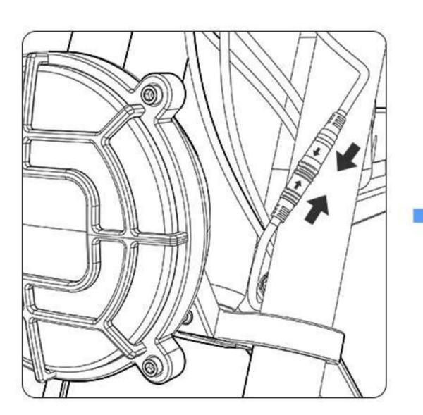
16. Plug in the headlight connector as per the directed arrow on it.
