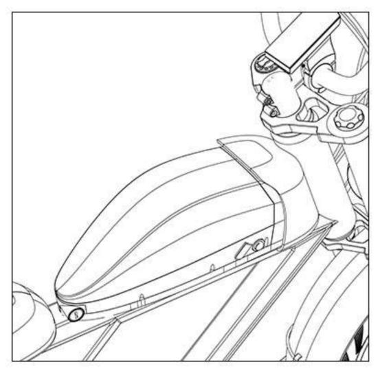
Push the battery inward horizontally to secure the battery into place.
