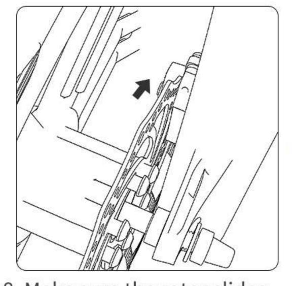
8. Make sure the rotor slides through in between the brake pads inside the caliper.
