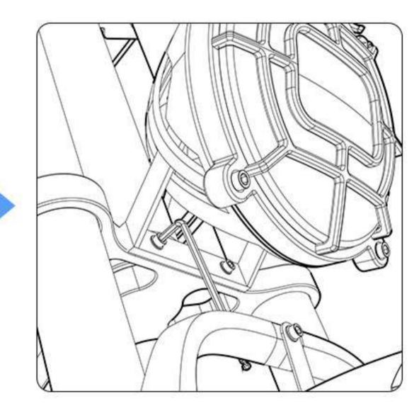
15. Attach the headlight to the front fork. Tighten the bolts with a 4mm Allen key.
