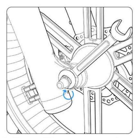
Use a 15mm open-end wrench to fully secure axle nuts.
