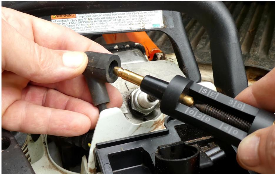
**STEP 3** Adjust the tester's screw to set a spark gap to 5mm (point A) on the tester for your 2-cycle small engine.
