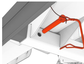
3. Insert the quick-release pin
