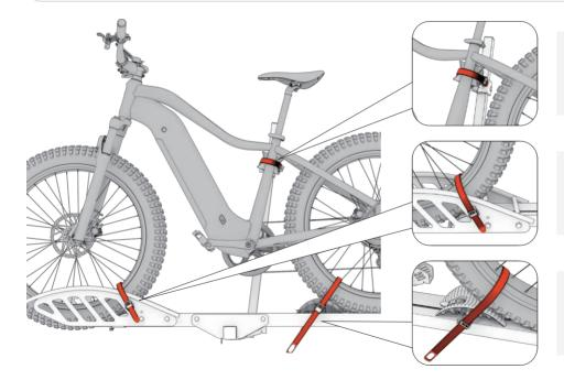
**Note:** Use the ratchet wheel strap to fix and tighten the seat tube or horizontal tube of the bicycle.
