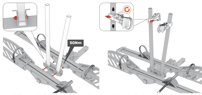
Insert Middle Support Tube (10) into the base of Bottom Fixing Bracket (2), then fix them with M10x60 Bolt (11) and M10 Lock Nut (9). Install the adjustable **Connecting Block (12)** to the **Middle Support Tube (10)**, then tighten the knob from the **Connecting Block (12)**.
