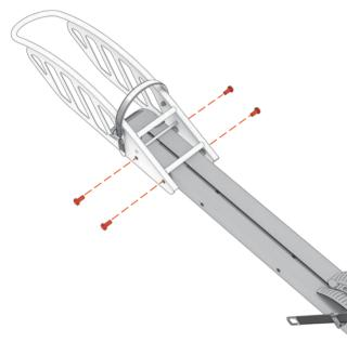
Align the holes from Front Wheel Holder (6) and Beam Assembly (5). Then fix them with M10\*20 Hex Bolt (7).
