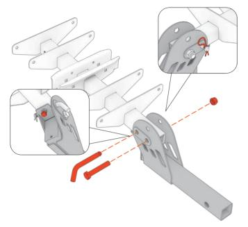
figure to eliminate the gap between the **Bottom fixing bracket (2)** and the **Rotating Group(1)**.
