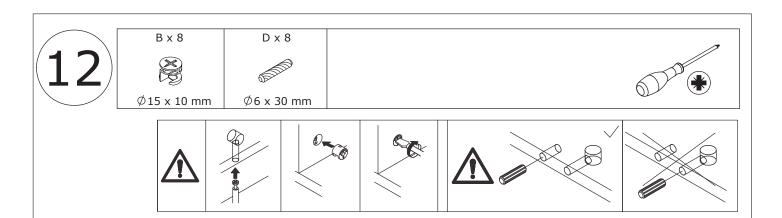
Connect the two components with wooden dowel(D) and turn cam lock(B) clockwise to tighten as shown.
