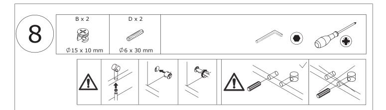
Attach No.9 plate to No.13 with wooden dowel(D) and turn cam lock(B) clockwise to tighten as shown.
