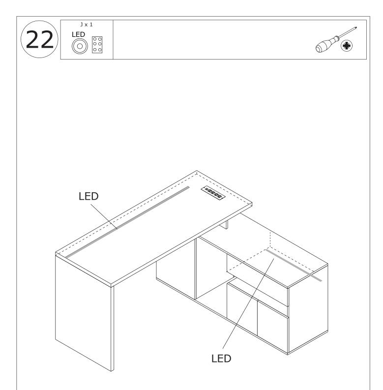
Stick light strip to back of board 1 and 12 at first. Use the remote to control the light strip or scan the QR code and download the APP to control.
