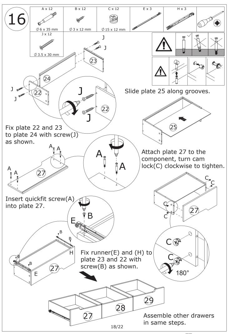
Align rails, slide drawers in corresponding positions.
