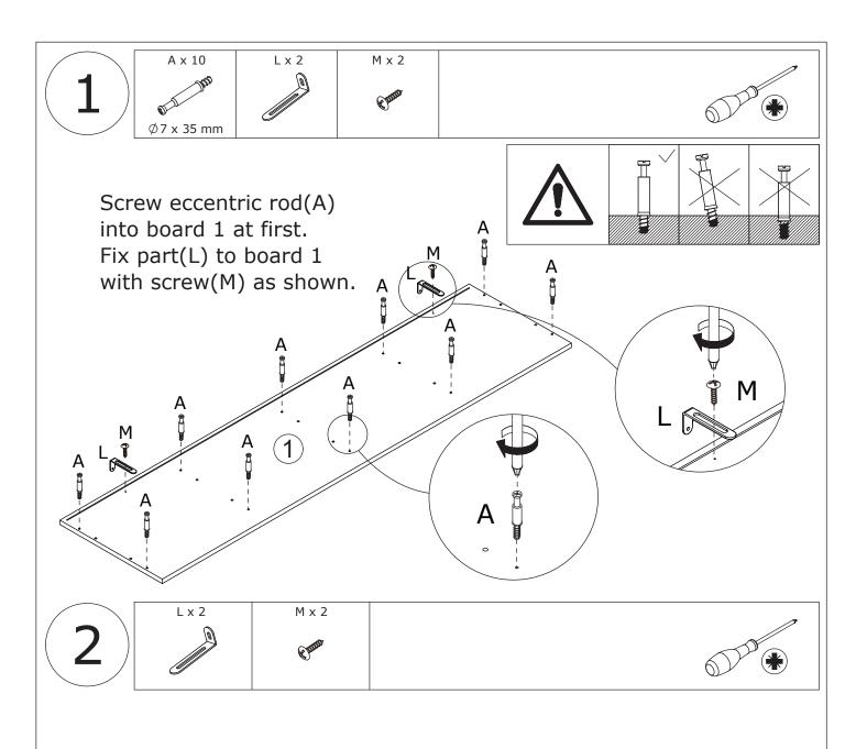
Fix part(L) to board 2 with screw(M) as shown.
