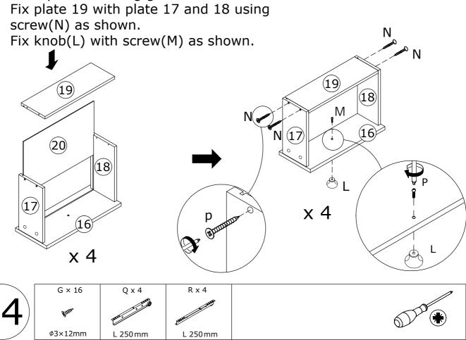
Fix runner(Q) and (R) to plate 17 and 18 respectively using screw(G) as shown.
