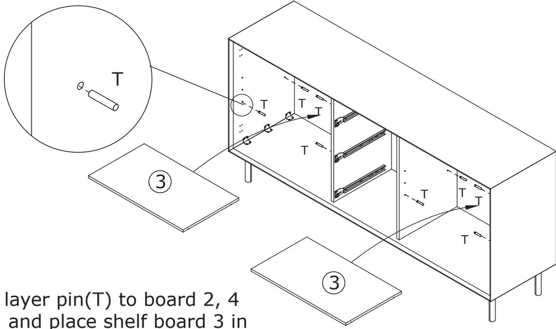
Insert layer pin(T) to board 2, 4 and 5, and place shelf board 3 in as shown.
