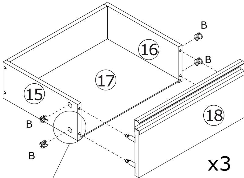
Connect board 18 to board 15 and 16, add cam lock(B) and turn clockwise to tighten as shown.
