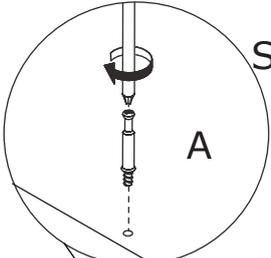
Screw eccentric rod(A) into board 1 with a screwdriver as shown.
