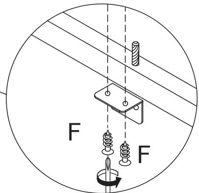
Fix board 6 to part(L) with screw(F) as shown.
