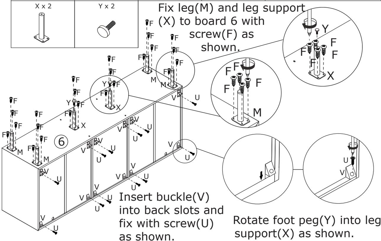
Insert buckle(V) into back slots and fix with screw(U) as shown.
