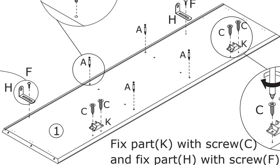
Fix part(K) with screw(C) and fix part(H) with screw(F) as shown.
