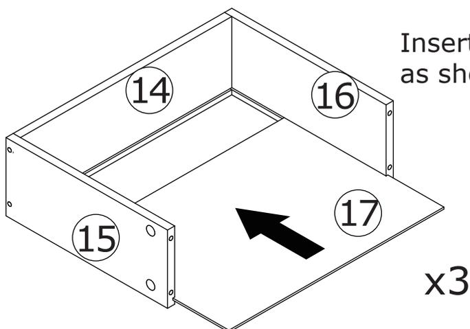
Insert bottom board 17 along grooves as shown.
