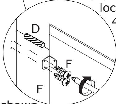
Fix board 1 to part(L) with screw(F) as shown.
