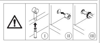
Attach plate 7 to plate 3; plate 6 to plate 2, add cam lock(B) into plate 6,7 and turn clockwise to tighten as shown.
