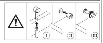
Attach plate 6 to plate 5, add cam lock(B) into plate 6 and turn clockwise to tighten as shown.
