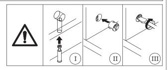
Attach plate 5 to plate 7 with screw(N), add cam lock(B) into plate 7 and turn clockwise to tighten as shown.
