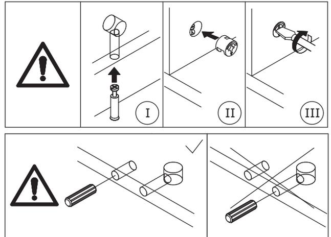
Knock LONG wooden dowel(J) into plate 7 and 8 at first.
