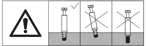
Insert quickfit screw(A) into corresponding holes in plate 1 with a screwdriver as shown.
