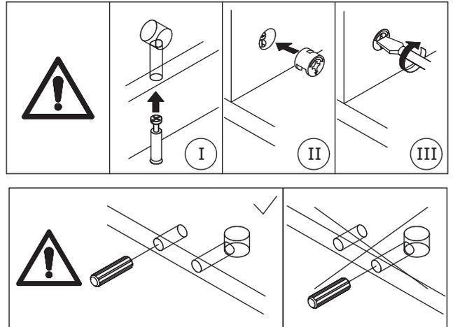
Attach another plate 7 and 8 to plate 5, add cam lock(B) into plate 7, 8 and turn clockwise to tighten as shown.
