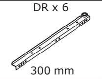
Fix runner(DL) and (DR) to plate 20 and 22 with screw(F) as shown.
