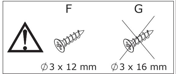
Fix slide rail(CL) to plate 5 with screw(F) at first.
