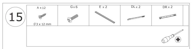
As shown in the picture, use the G screw to connect the E handle to the 17 drawer plate; Fix the slide DL and DR To the bottom of the drawer using screw No. C.
