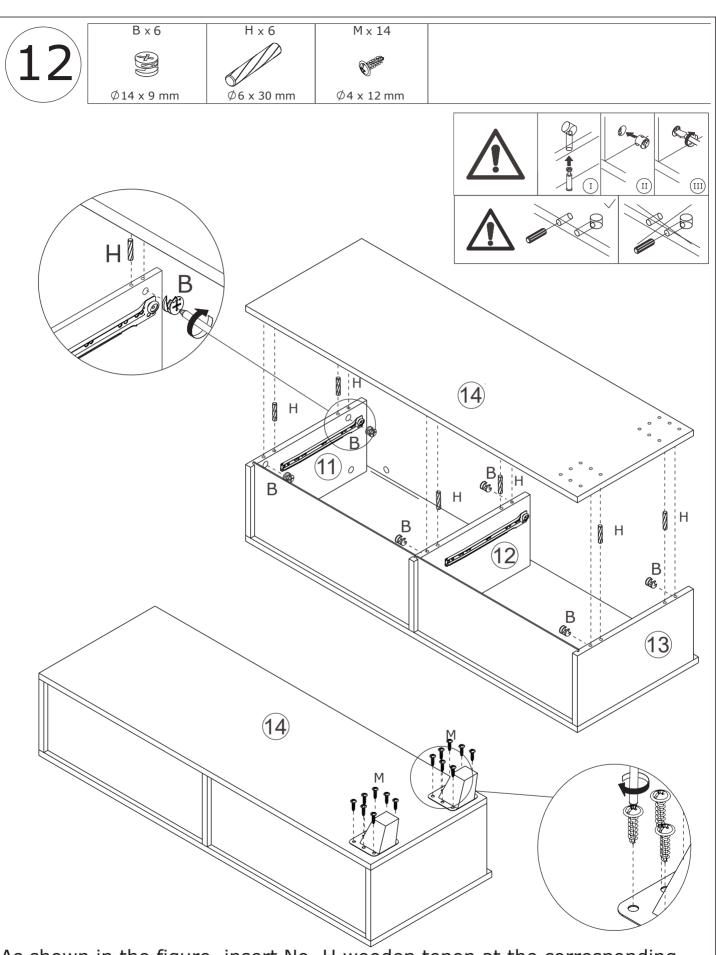
As shown in the figure, insert No. H wooden tenon at the corresponding reserved holes on No. 11, No. 12 and No. 13 plates, cover No. 14 plate, and put in No. B eccentric wheel to rotate 90-180 degrees clockwise; Finally, connect the foot of the TV cabinet to the cabinet body with the M screw.
