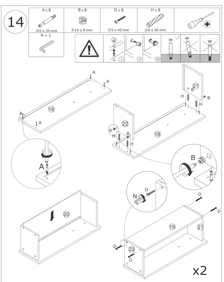
As shown in the picture, fix No. A screw and No. H wooden tenon No. 18, insert No. 21 and No. 22 plates, put in No. B eccentric wheel and rotate clockwise 90-180 degrees; Then insert No. 20 sheet and connect No. 19 plate to No. 21 and No. 22 plate using No. D screw and No. N wrench.
