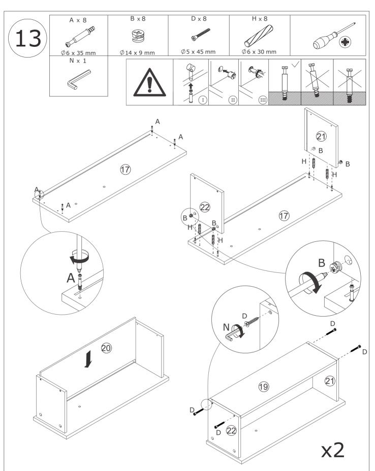
As shown in the picture, fix No. A screw and No. H wooden tenon No. 17, insert No. 21 and No. 22 plates, put in No. B eccentric wheel and rotate clockwise 90-180 degrees; Then insert No. 20 sheet and connect No. 19 plate to No. 21 and No. 22 plate using No. D screw and No. N wrench.
