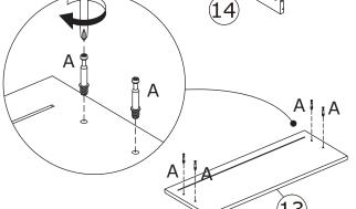
Insert quickfit screws A to board 13 as shown.
