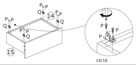
Fix casters Q on boards 14 and 15 by using screws P as shown.
