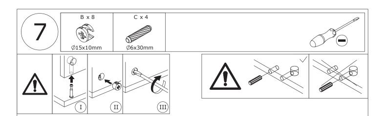
Insert wooden dowels C into boards 1 and 9 as shown, then attach board 6 to assembled unit, insert cam locks B into the corresponding holes of boards 1,2,4 and 9, turn cam locks clockwise to tighten as shown.
