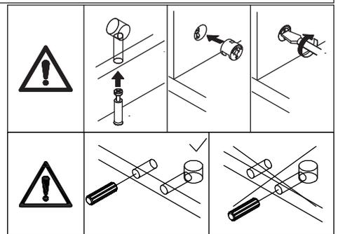
Attach plate 4 to plate 8 with wooden dowel(D) at first. Put cam lock(C) into holes in plate 4 and turn clockwise to tighten as shown.
