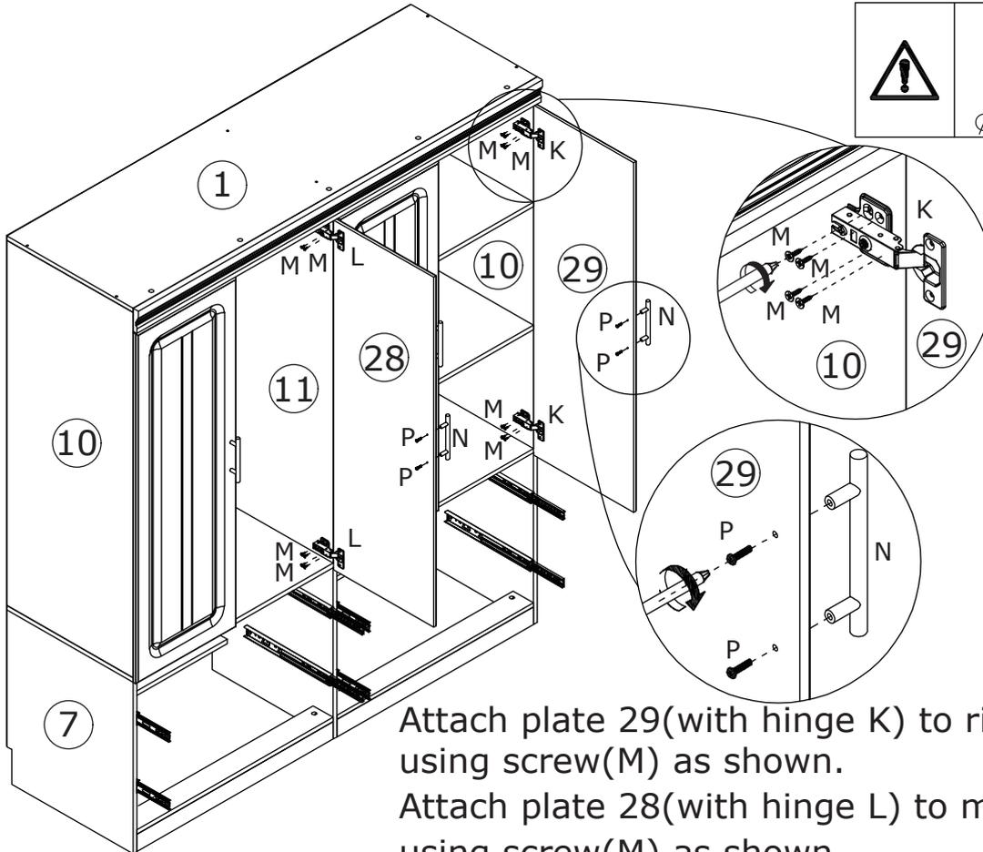
Attach plate 29 (with hinge K) to right side plate 10 using screw (M) as shown.
