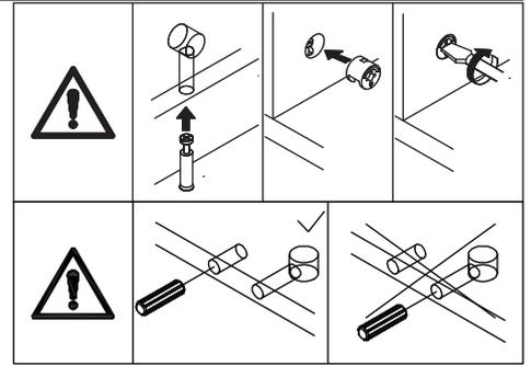
Attach plate 3 and 15 to plate 7 with wooden dowel(D) at first. Put cam lock(C) into holes in plate 3 and turn clockwise to tighten as shown.
