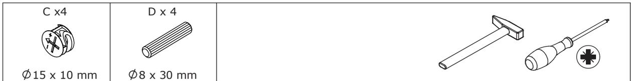
Attach plate 20 to plate 18 with wooden dowel(D) at first.
