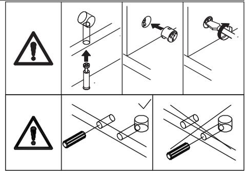
Attach plate 2 and 14 to plate 8 with wooden dowel(D) at first. Put cam lock(C) into holes in plate 2 and turn clockwise to tighten as shown.
