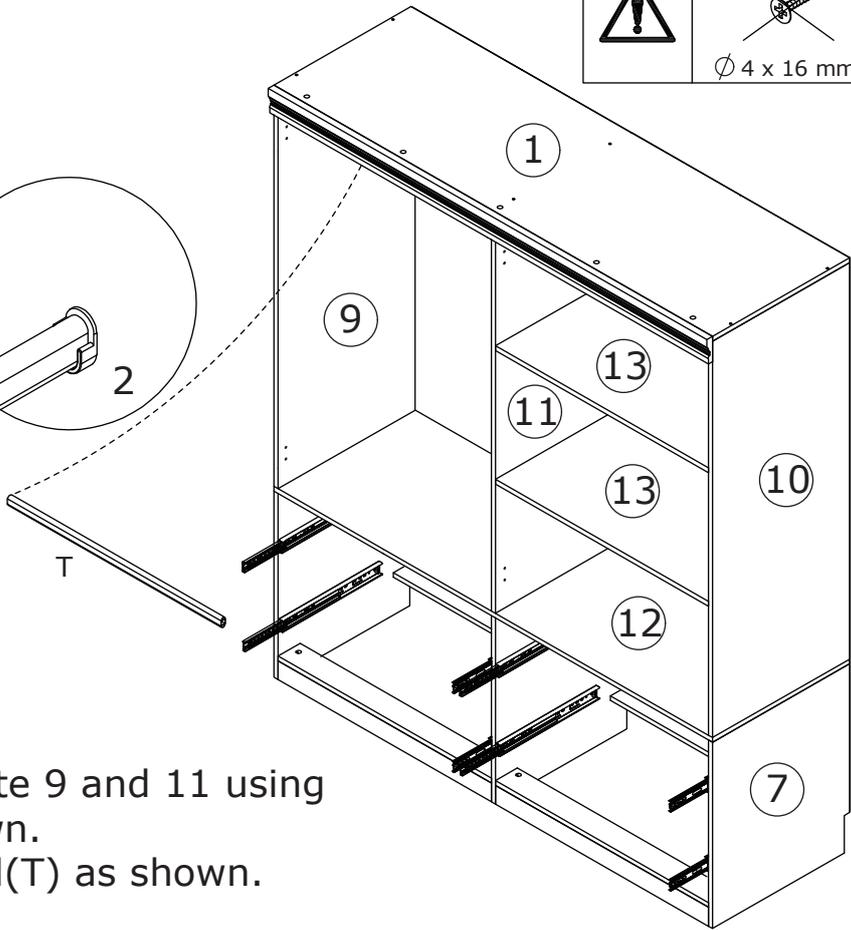
Fix part(S) to plate 9 and 11 using screw(U) as shown.
