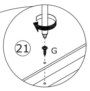
Fix back plate 21,22,23,24,25 and 26 using screw(G) at first. Fix each plate together using iron sheet(H) with screw(J) as shown.
