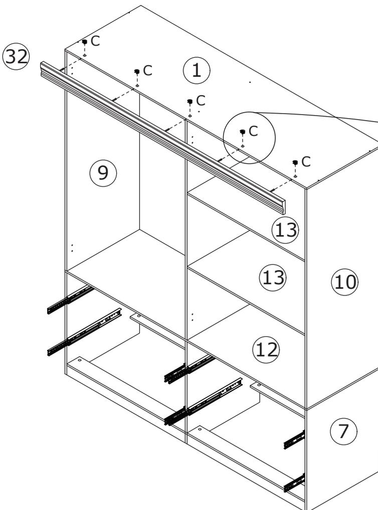
Attach plate 32 to plate 1 at first.
