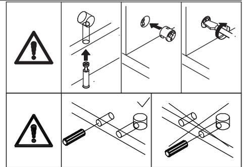
Attach plate 5 to plate 7 with wooden dowel(D) at first. Put cam lock(C) into holes in plate 5 and turn clockwise to tighten as shown.
