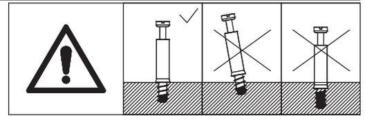
Insert quickfit screw(A) into corresponding holes in plate 11 with a screwdriver as shown.
