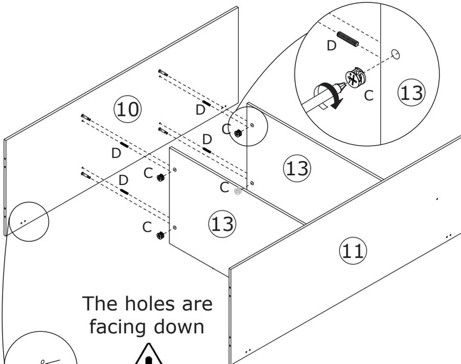
Attach plate 10 to plate 13 with wooden dowel(D) at first.
