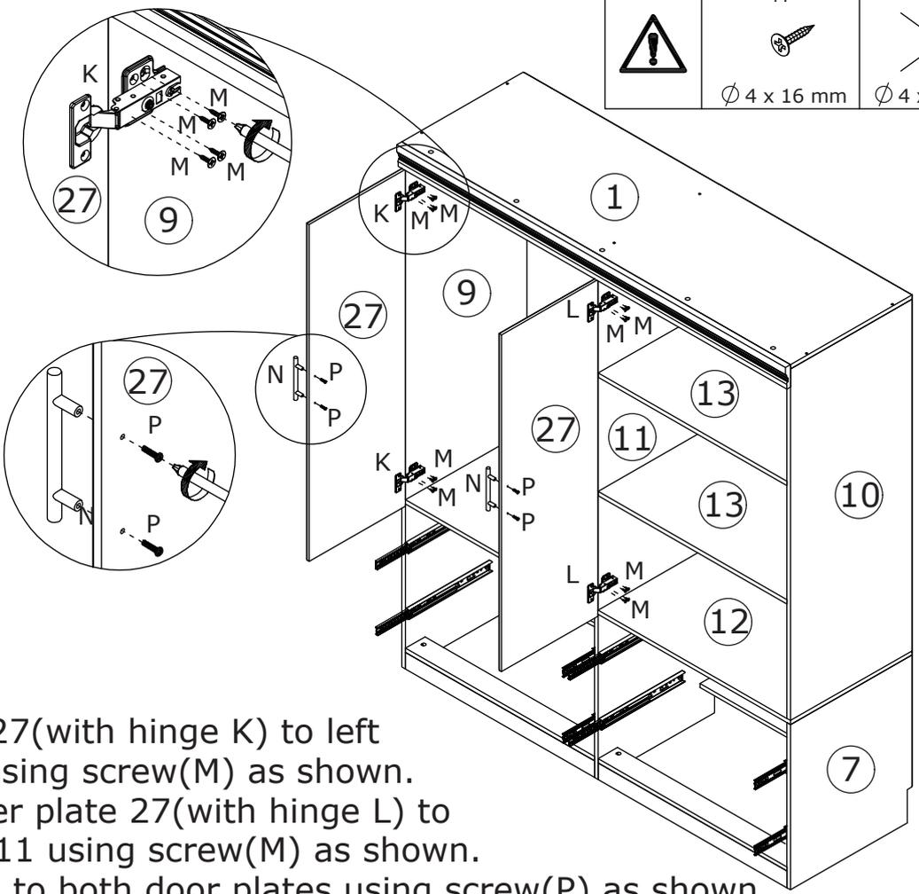
Attach plate 27(with hinge K) to left side plate 9 using screw(M) as shown.
