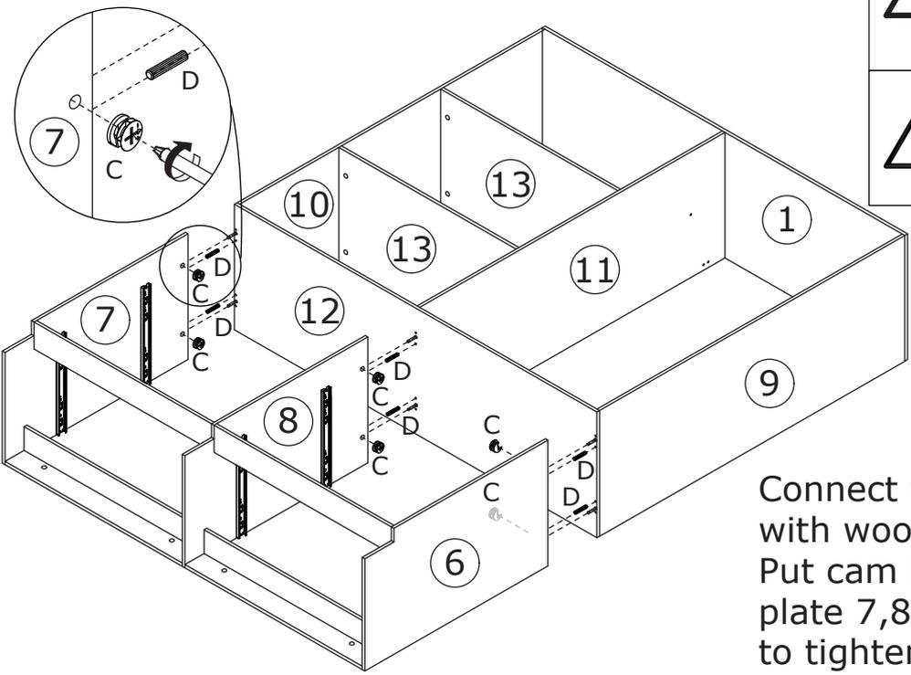
Connect the two components with wooden dowel(D) at first. Put cam lock(C) into holes in plate 7,8,6 and turn clockwise to tighten as shown.
