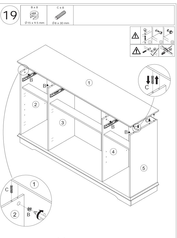
Insert wooden dowel(C) into board 2,3,4,5at first. Attach board 2,3,4,5 to board 1 add cam lock(B) into board 2,3,4,5 and turn clockwise to tighten as shown.
