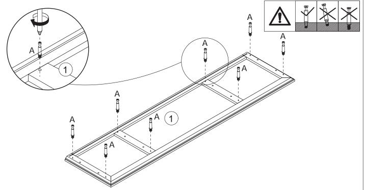
Screw eccentric rod(A) into board 1 with a screwdriver as shown.
