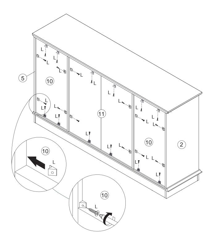
Insert buckle(L) into back slots and fix with screw(L) as shown.
