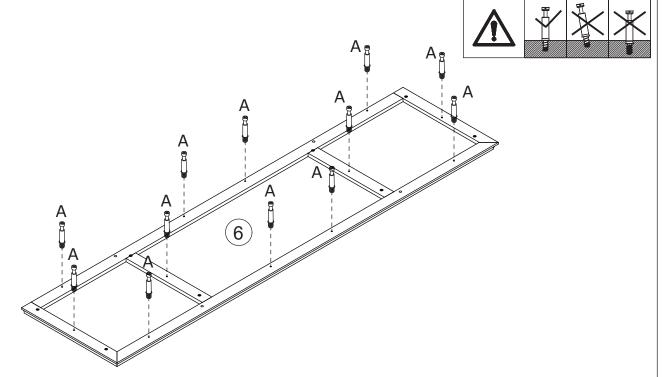
Screw eccentric rod(A) into board 6 with a screwdriver as shown.
