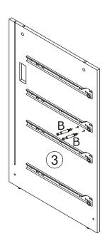
Insert quickfit screw(B) into corresponding holes in board 2,3,4 with a screwdriver as shown.
