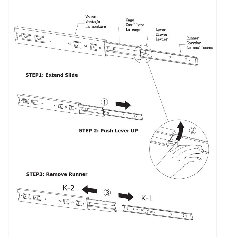
Separate glides(K) into two parts as shown.
