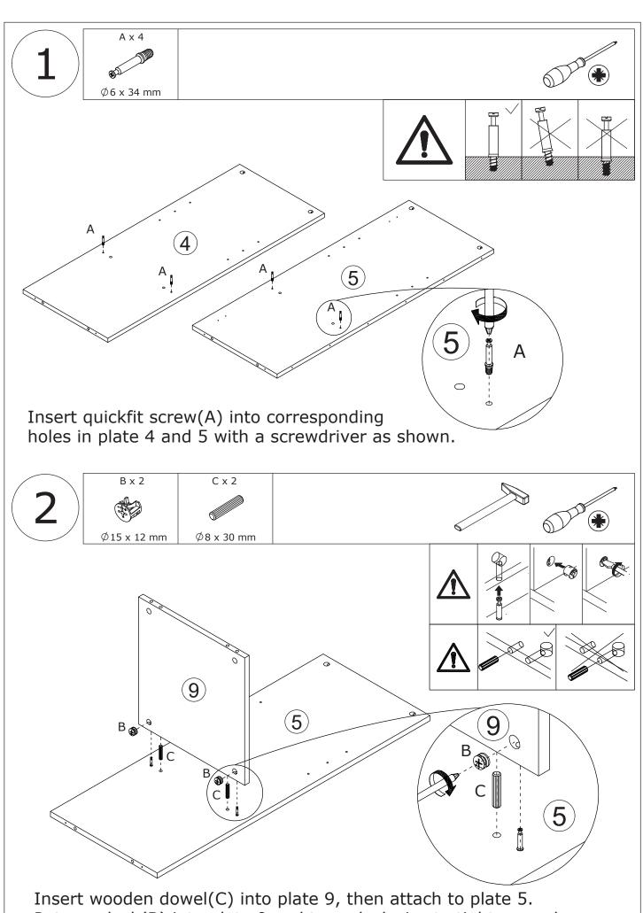
Insert wooden dowel(C) into plate 9, then attach to plate 5. Put cam lock(B) into plate 9 and turn clockwise to tighten as shown.
