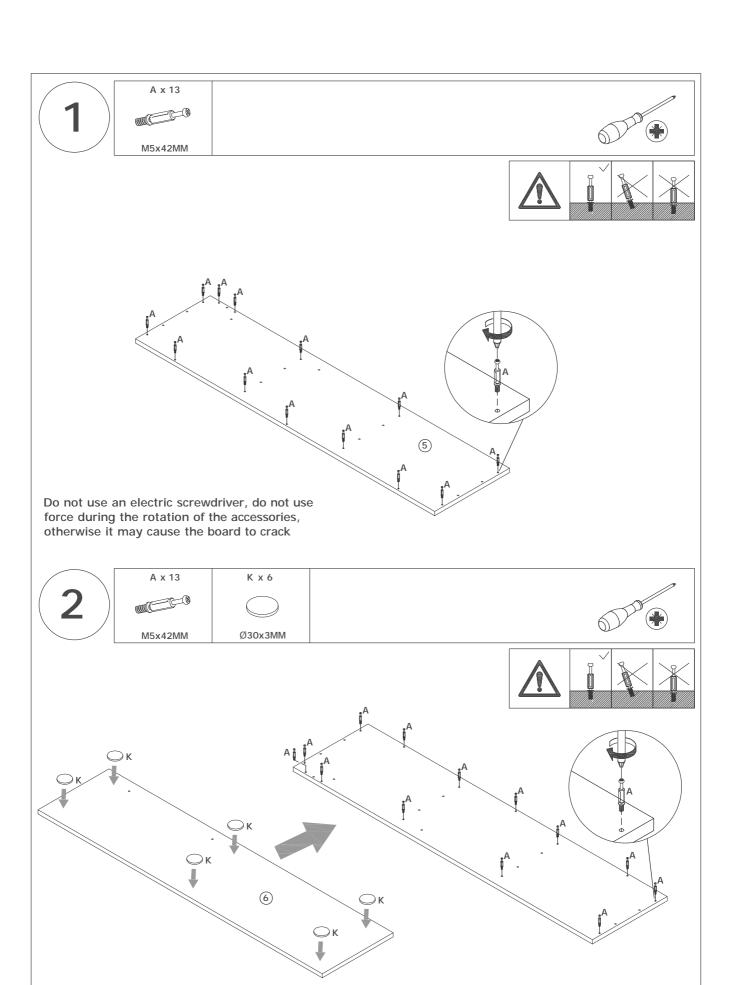
Do not use an electric screwdriver, do not use force during the rotation of the accessories, otherwise it may cause the board to crack
