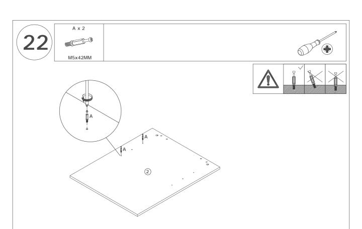
Do not use an electric screwdriver, do not use force during the rotation of the accessories, otherwise it may cause the board to crack
