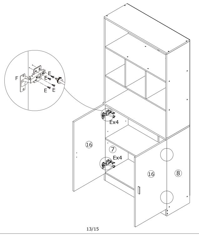
If there is misalignment after you install, adjust the screw to the best condition.
