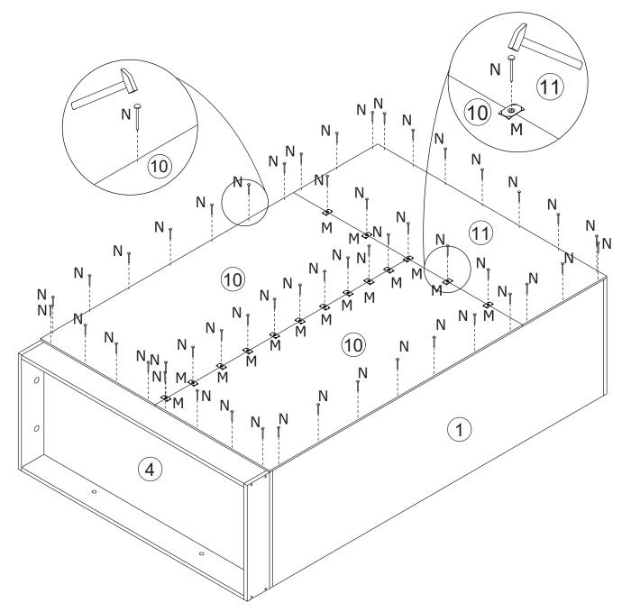
Fix back board 11 and 10 to the component with nail(N) at first. Use iron sheet(M) to fix board 10 and 11 with nail(N) as shown.
