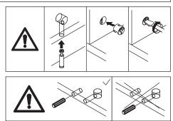
Attach board 6 to board 4 using wooden dowel(C), add cam lock(B) into board 6 and turn clockwise to tighten as shown.
