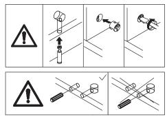
Connect board 4 to board 2 and 3 using wooden dowel(C), add cam lock(B) into board 4 and turn clockwise to tighten as shown.
