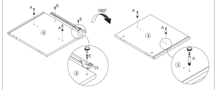
Screw eccentric rod(A) into board 5 and fix slide rail(CR) with screw(E) at first.
