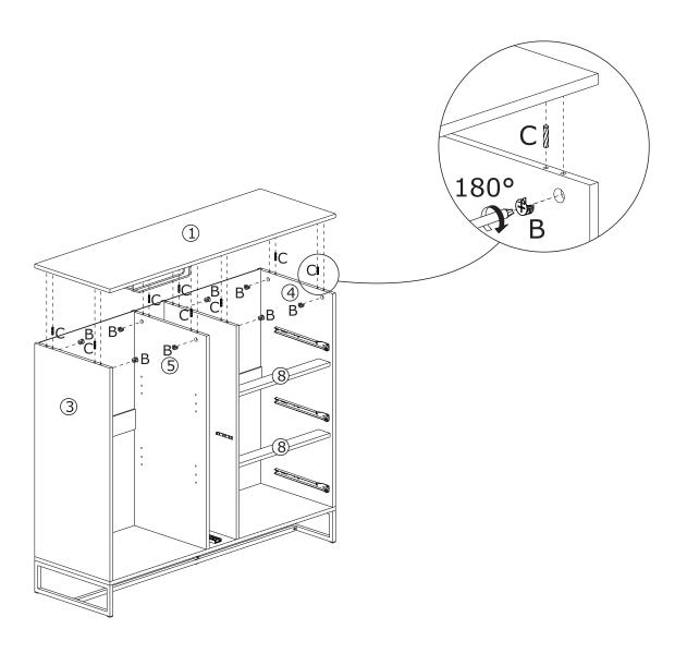
Cover board 1 to the component using wooden dowel(C), add cam lock(B) into board 3,5,6,4 and turn clockwise to tighten as shown.
