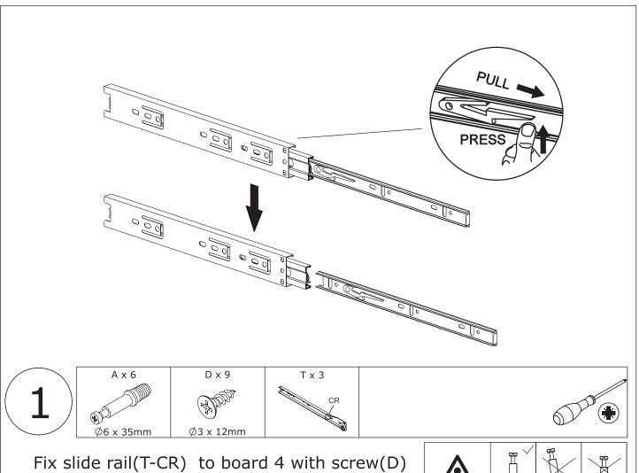
Fix slide rail(T-CR) to board 4 with screw(D) as shown.
