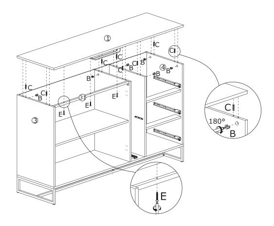
Cover board 1 to the component using wooden dowel(C), add cam lock(B) into board 3,5,6,4 and turn clockwise to tighten as shown.
