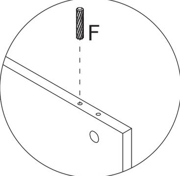
Insert wooden dowels(F) to the corresponding holes in No.2 and No.3 plate slightly.
