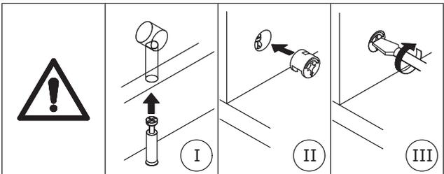
Cover No.1 to No.2 and No.3 plate, turn cam lock(E) clockwise to tighten as shown.
