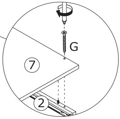
Cover No.7 to No.2 and No.3 plate with screw(G) as shown.
