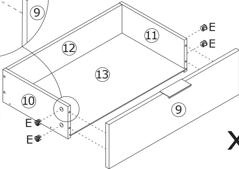
Attach No.9 plate and turn cam lock(E) clockwise to tighten as shown.
