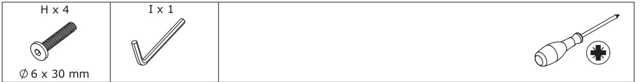
Fix leg 8 to No.7 plate with screw(H) as shown.
