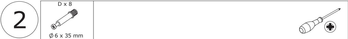
Insert quickfit screw(D) into No.2 and No.3 plates as shown.
