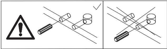
Insert wooden dowels(F) to the corresponding holes in No.2 and No.3 plate slightly. Slide No.6 plate to the available slots as shown.
