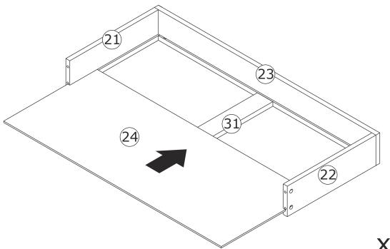
Insert bottom board 24 along available grooves as shown.
