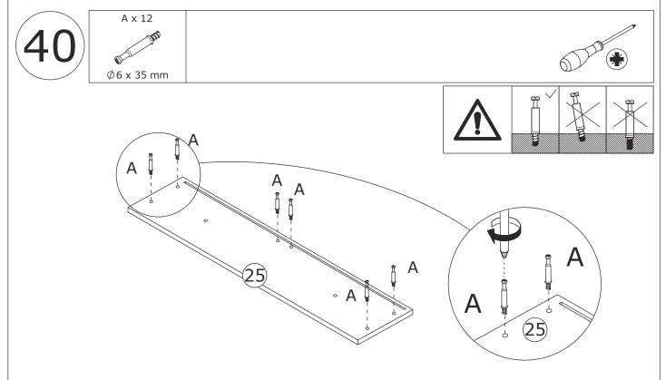
Screw eccentric rod(A) into board 25 at first.
