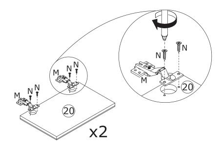
Fix hinge (M) to plate #20 with screw(N) as shown.
