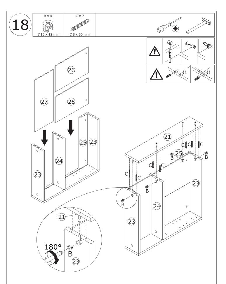
Slide plate #26/#27 into available slots, fix plate #21 to plate #23/#24/#25 using wooden dowel(C) and inserting cam lock (B) into plate #7/#8, and turn clockwise to tighten as shown.
