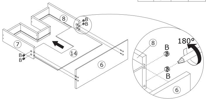
Slide plate #14 into available slots as shown. Fix plate #6 to plate #7/#8 by insert cam lock(B) into plate #7/#8 and turn clockwise to tighten as shown.
