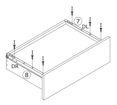
Using screw(I) to lock runner(DL) and (DR) to plate #7/#8 as shown.
