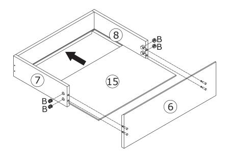
Slide plate #15 into available slots as shown. Fix plate #6 to plate #7/#8 by insert cam lock(B) into plate #7/#8 and turn clockwise to tighten as shown.
