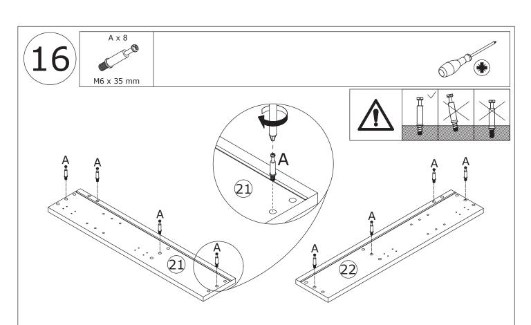
Insert quickfit screw(A) into corresponding holes in plate #21/#22 with a screwdriver as shown.
