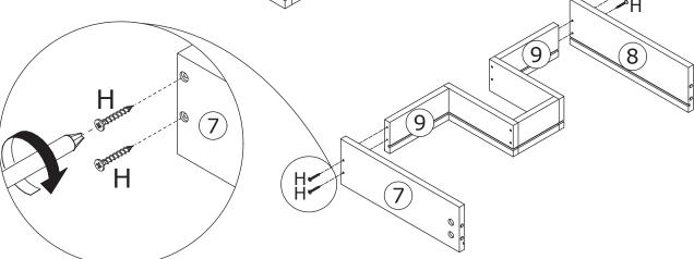
Connect plate #7/#8 to plate #9 of the component (assembled in step 5) using screw(H) as shown.
