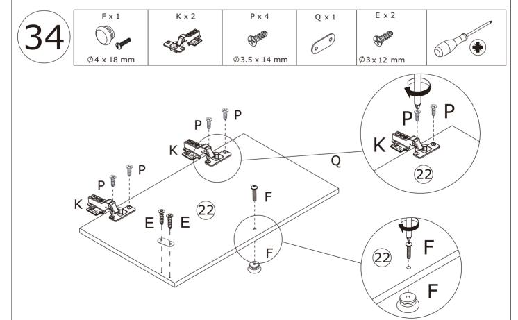
Fix hinge(K) to board 22 with screw(P) as shown.
