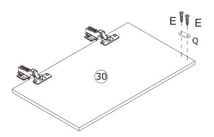
Fix part(Q) to board 30 with screw(E) as shown.
