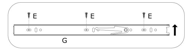
Separate glide into two parts at first.
