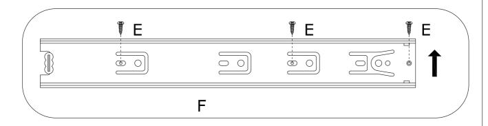
Fix slide rail(F) to board 1 with screw(E) as shown.
