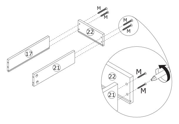
Fix board 22 to board 17 and 21 using screw(M) as shown. Insert bottom board 23 along available grooves as shown.
