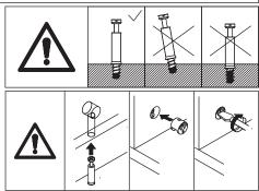
Screw eccentric rod(A) into board 24 as shown. Attach board 24 to board 17 and 21, add cam lock(B) into and turn clockwise to tighten as shown.
