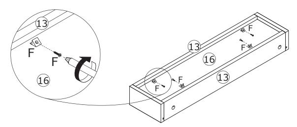
Place board 15 into the part, flip to back. Insert buckle(F) into back slots and fix to tighten as shown.
