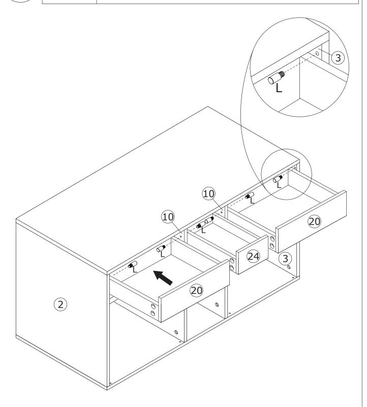
Insert layer pin(L) into board 2, 10 and 3 as shwon.
