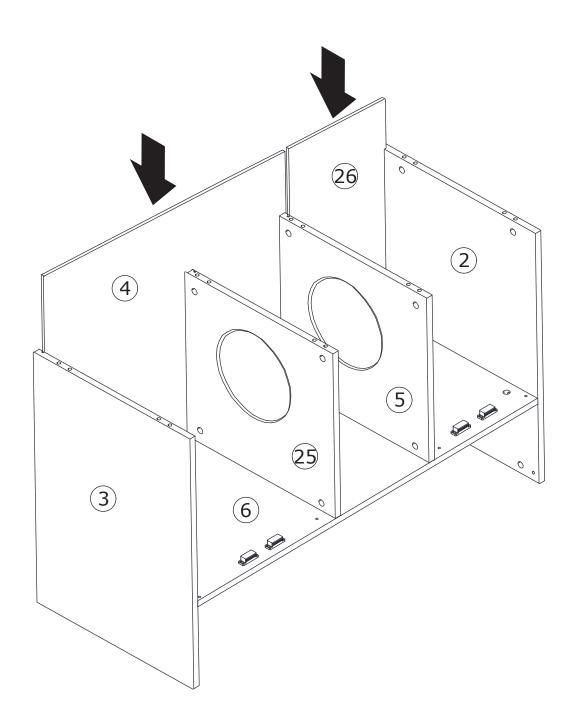
Insert back board 4 and 26 along available grooves as shown.
