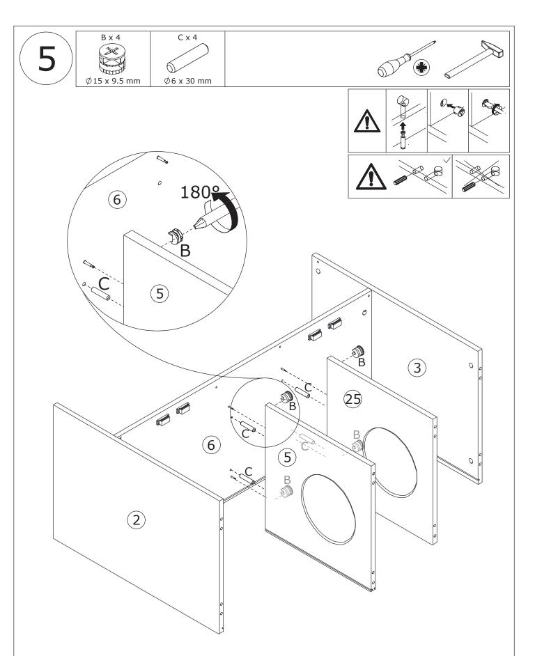
Attach board 5 and 25 to board 6 using wooden dowel(C), add cam lock(B) into board 5,25 and turn clockwise to tighten as shown.
