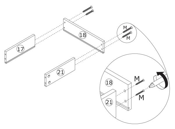
Fix board 18 to board 17 and 21 using screw(M) as shown. Insert bottom board 19 along available grooves as shown.
