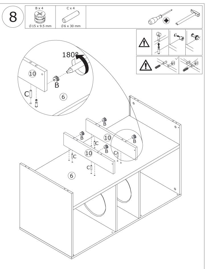
Attach board 10 to board 6 using wooden dowel(C), add cam lock(B) into board 10 and turn clockwise to tighten as shown.
