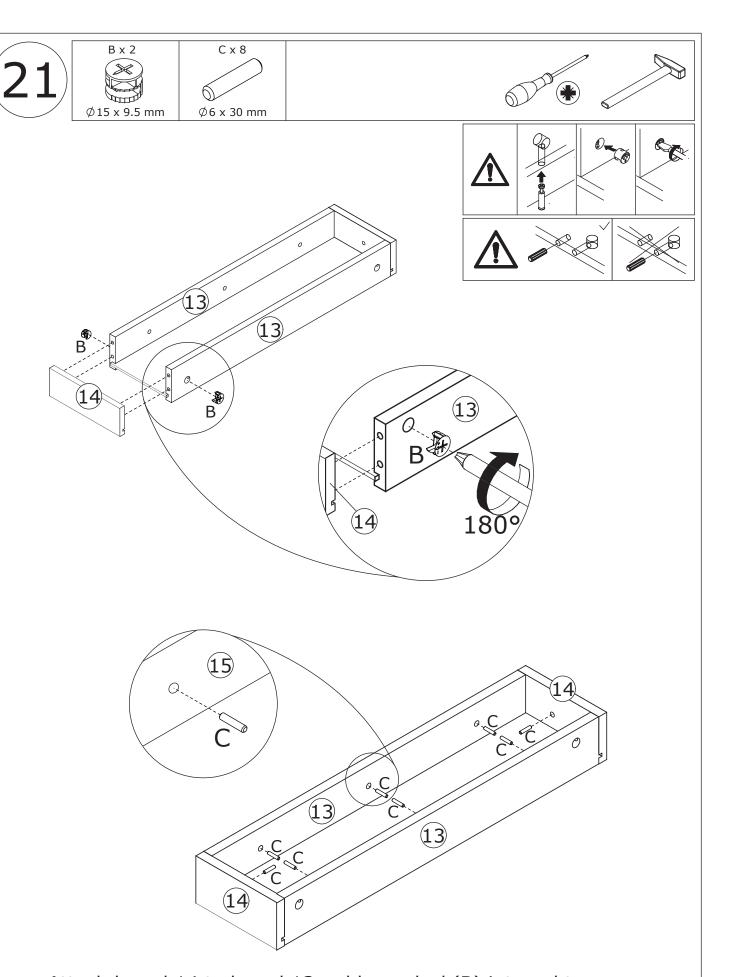
Attach board 14 to board 13, add cam lock(B) into and turn clockwise to tighten as shown.
