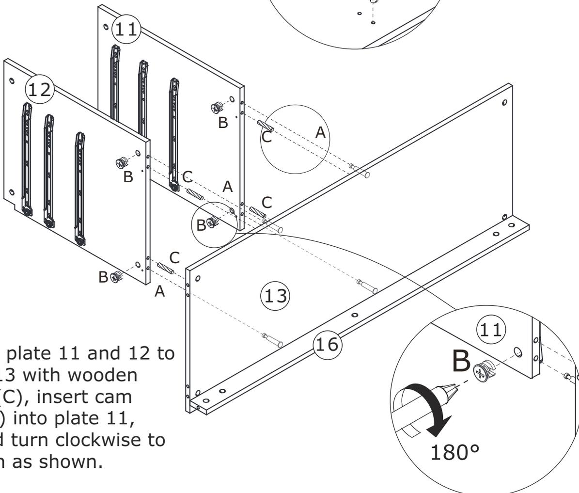
Attach plate 11 and 12 to plate 13 with wooden dowel(C), insert cam lock(B) into plate 11, 12 and turn clockwise to tighten as shown.
