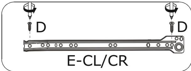
Fix slide rail(E-CL) to plate 12 using screw(D) as shown. Flip the plate, fix slide rail(E-CR) using screw(D) as shown.
