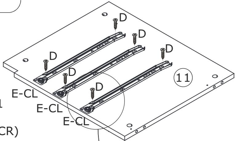
Fix slide rail(E-CL) to plate 11 using screw(D) as shown. Flip the plate, fix slide rail(P-CR) using screw(D) as shown.
