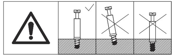
Insert quickfit screw(A) into corresponding holes in plate 8 as shown.
