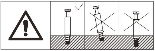
Insert quickfit screw(A) into corresponding holes in plate 20,21 and 24 with a screwdriver as shown.
