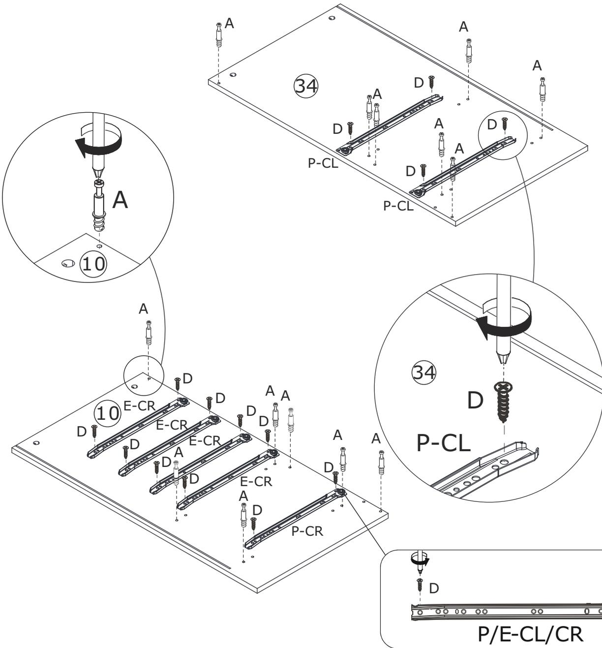
Fix slide rail(P-CL) to plate 34 using screw(D) as shown.
