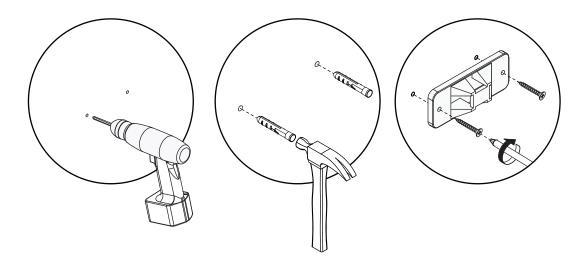
Install anti-tipping device as shown.
