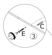
Using screw(E) and dowel(C) to connect panel #5 with panel #3 as shown.
