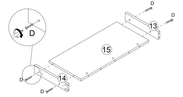
Using screw(D) to connect panel#13,#14 with panel#15 as shown.
