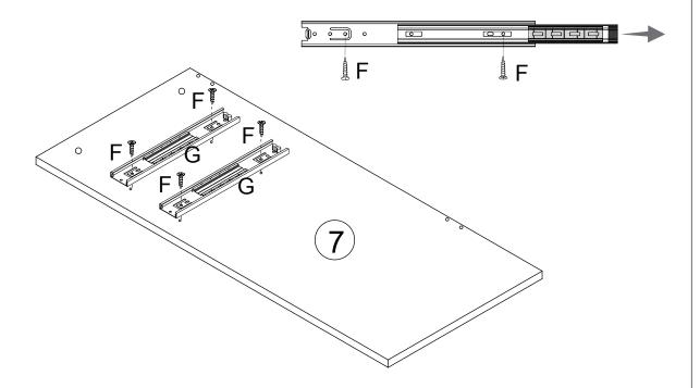
Using screw(F) to lock the silde(G) to the panel #7as shown.
