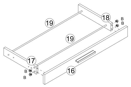
Connect panel#19 with panel#17,#18, Connetc panel#16 with panel#17,#18 and insert the lock(B) to the panel#17,#18 as shown.
