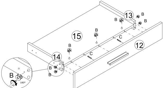
Using dowel(C) to connect panel #12 with panel #13, #14, #15 and insert the lock(B) to the panel #13, #14 as shown.
