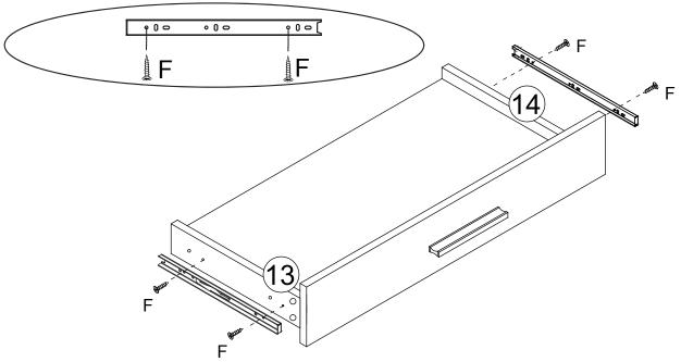
Using screw(F) to lock the slide to panel#13, #14 as shown.
