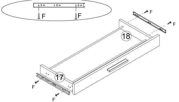
Using screw(F) to lock the slide to panel#17, #18 as shown.
