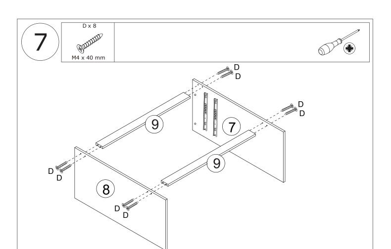
Using screw(D) to connect panel #9 with panel #7, #8 as shown.
