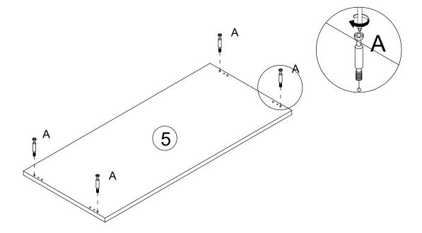
Insert cam bolt (A) to panel #5 as shown.
