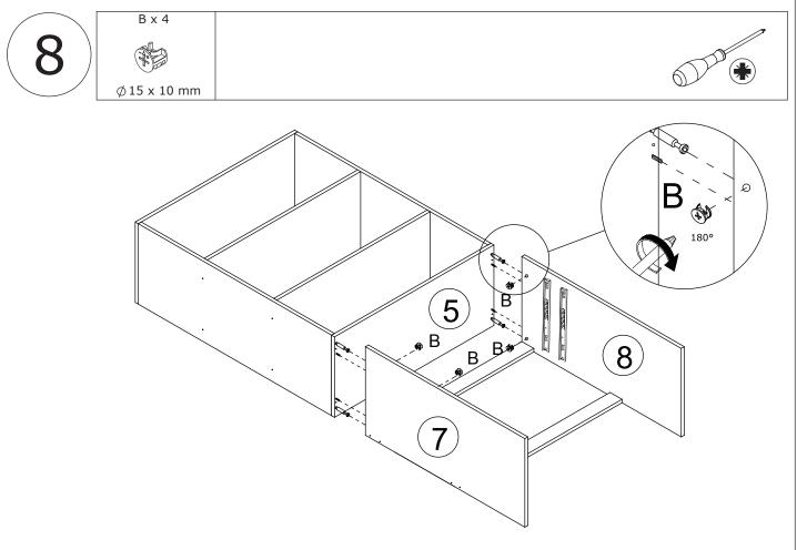
Connect panel #5 with panel #7, #8 and insert the lock(B) to the panel #7, #8 as shown.  $$_{9/17}$$
