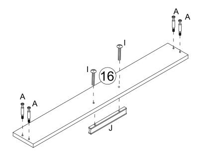
Insert bolt(A) to the panel #16, Using screw(I) to lock the handle(J) to the panel #16 as shown.
