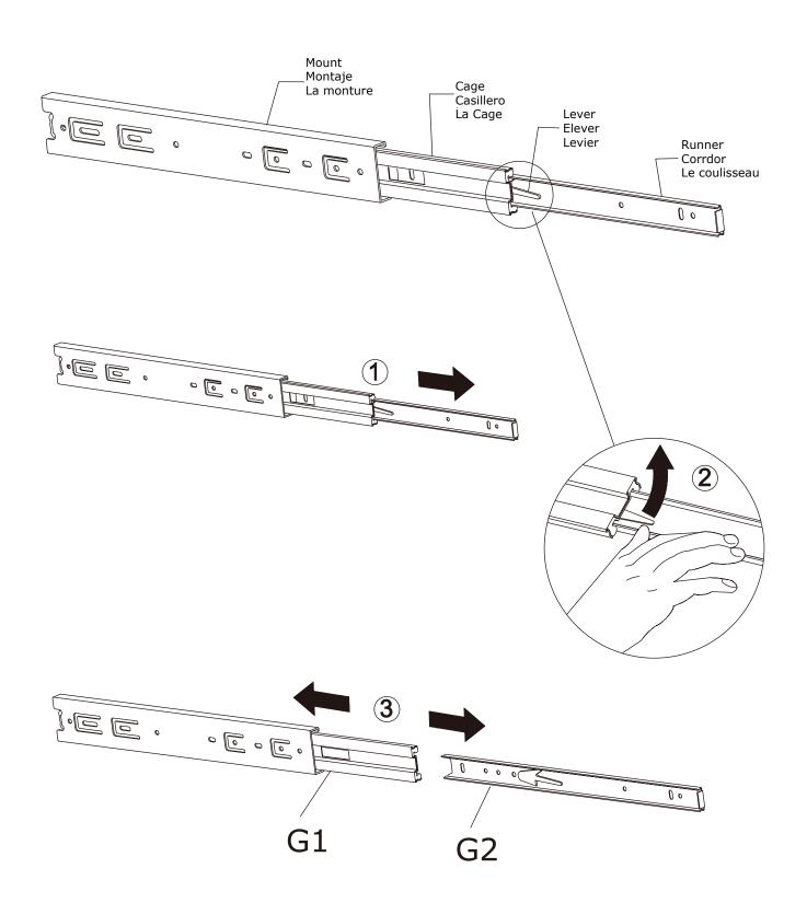
Separate glides(G) into two parts as shown.
