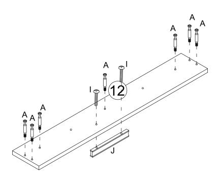
Insert bolt(A) to the panel #12, Using screw(I) to lock the handle(J) to the panel #12 as shown.
