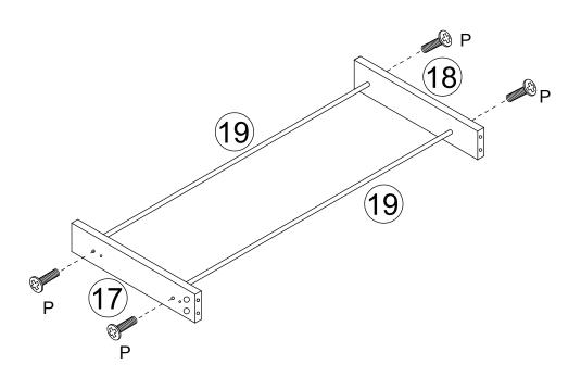
Using screw(P) to connect panel#19, with panel#17,#18 as shown.
