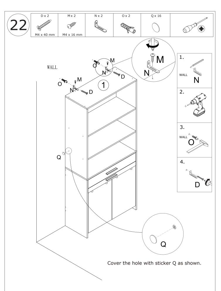
Using screw (M) to lock the L metal (N) to the top panel#1 as shown. Drill holes on wall, knock part(O) into the holes. Install anti-tipping device as shown.
