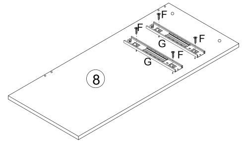
Using screw(F) to lock the silde(G) to the panel #7as shown.
