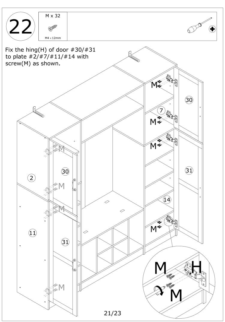
Adjust hinge screws to make door alignment. 22/23
