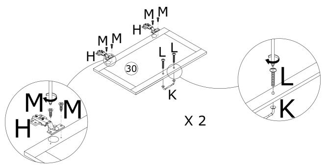
Fix the handle (K) to door #30/#31 with screw(L)as shown.
