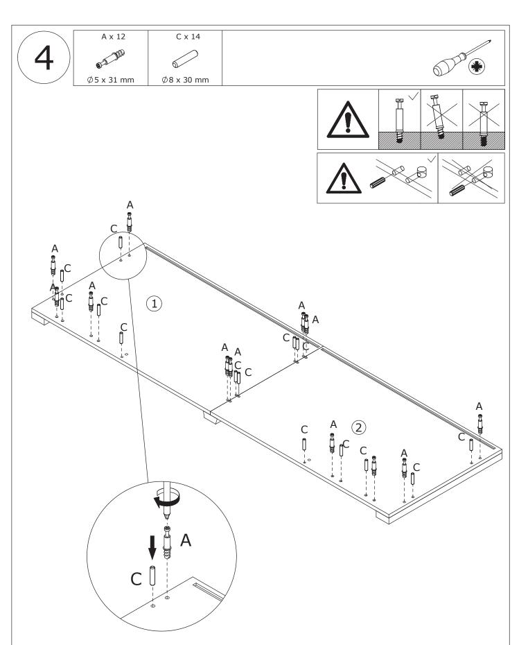
Flip the componet, screw eccentric rod(A) and insert wooden dowel(C) into board 1 and 2 as shown.
