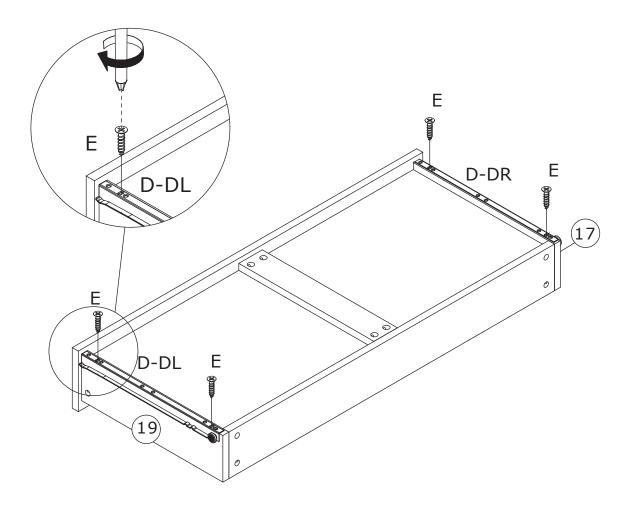
Fix runner(D-DL) and (D-DR) to board 19 and 17 with screw(E) as shown.
