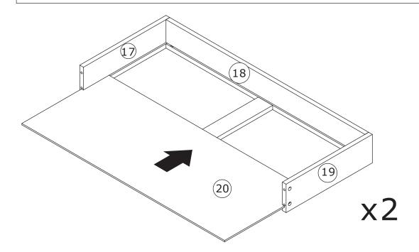
Insert bottom board 20 along available grooves as shown.
