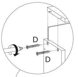
Insert board 28, 29, 34 and 35 along available grooves as shown.
