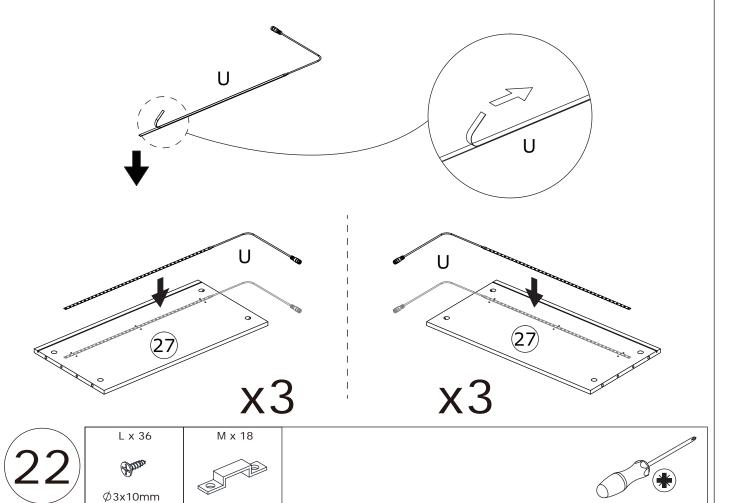
Fix light strip(U) to board 27 through buckle(M) and screw(L) as shown.
