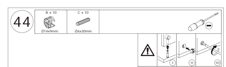
Attach board 35 to board 27, 28 and 29 using wooden dowel(C), add cam lock(B) into and turn clockwise to tighten as shown.
