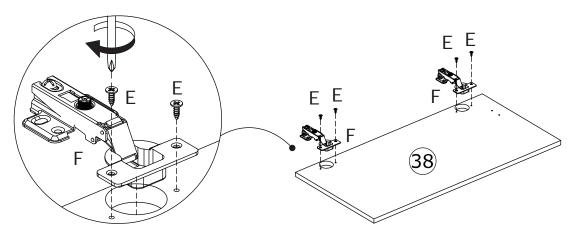
Assemble door 38 to board 20 by fixing hinge with screw(E) as shown.
