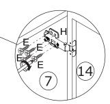
Assemble door 14 to board 6 and 7; door 15 to board 1; door 16 to board 2 by fixing hinge with screw(E) as shown.
