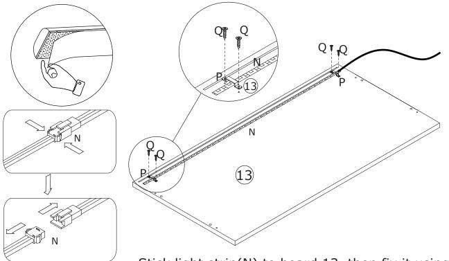
Stick light strip(N) to board 13, then fix it using part(P) and screw(Q) as shown.
