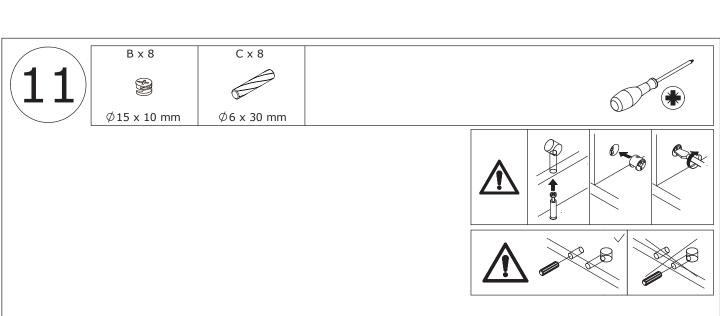
Knock wooden dowel(C) into plate 1, 2, 3 and 4 at first, then attach plate 5 to.
