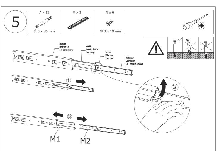
Fix slide rail(M1) to plate 3 and 4 with screw(N) as shown.
