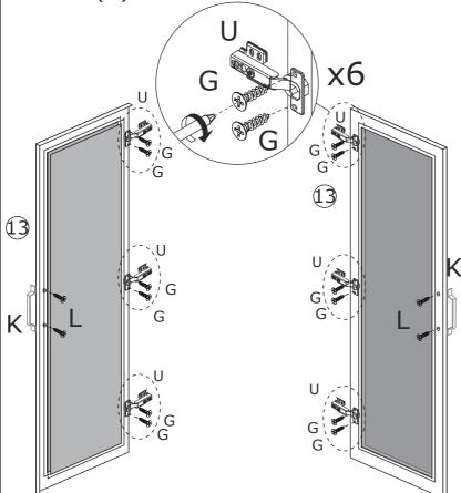
Fix handle(K) to door plate with screw(L) as shown.
